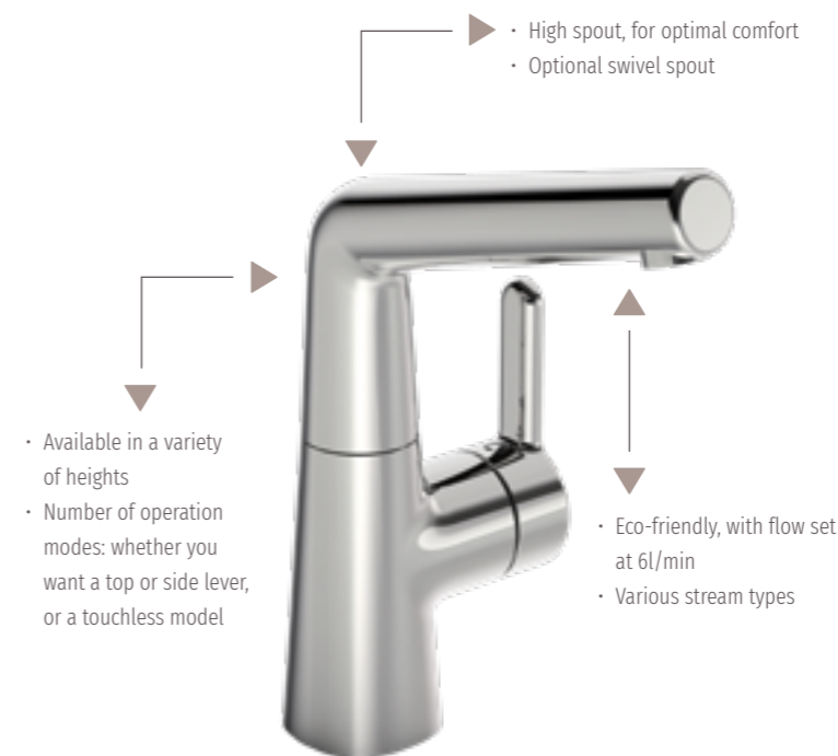
Single-lever mixer for washbasins, top-controlled, XL variant, bidet variant top operated
